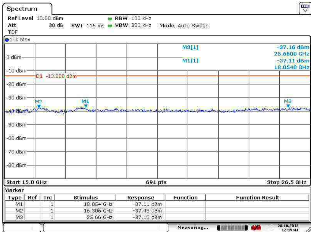
Figure 51. Mid channel conductive emission 15 GHz to 26.5 GHz (1 Mbps).
