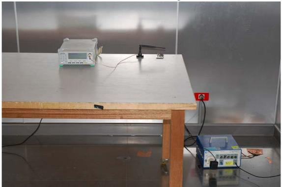
**Conducted Emission Set up Photo**
