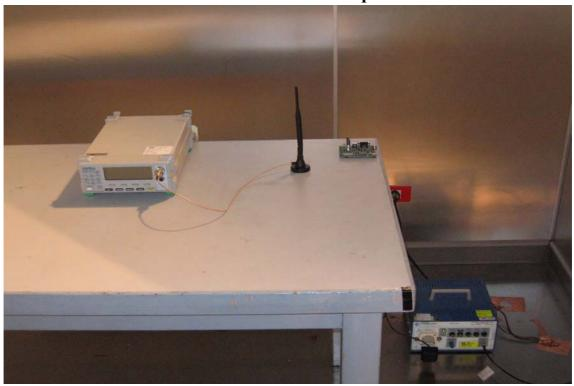
**Conducted Emission Set up Photo**
