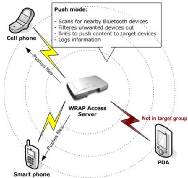
Figure 5-2. Obexsender Use Case: Content Push
