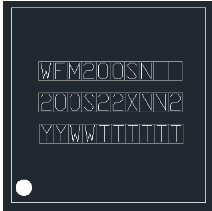
Figure 4: Top shield markings of WFM200SN
