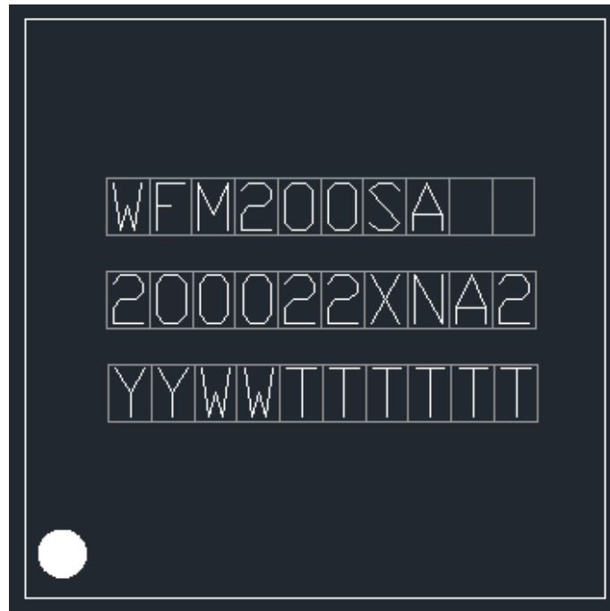
Figure 3: Top shield markings of WFM200SA
