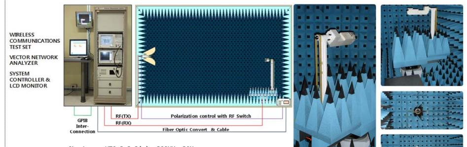
Chamber - MTG 6x3x3(m), 300MHz~6GHz Active - Agilent E5515C (8960 Series 10) Passive - Agilent E5071B 300KHz~8.5GHz
