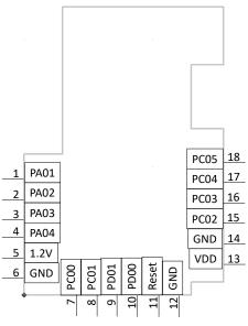
Figure 5: MGM210L pinout
