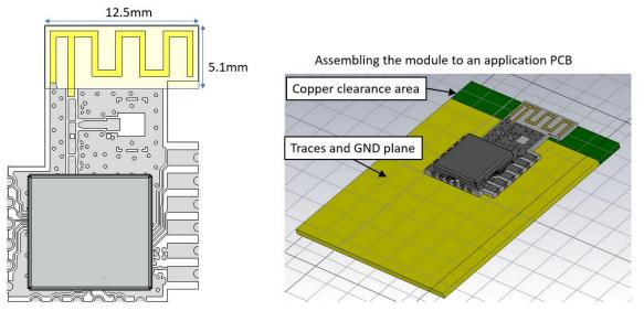
Figure 1: Installing the module to an application PCB
