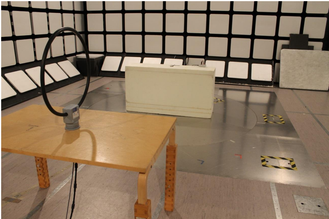
Photograph 2. Radiated Spurious Emissions 9 kHz - 30 MHz
