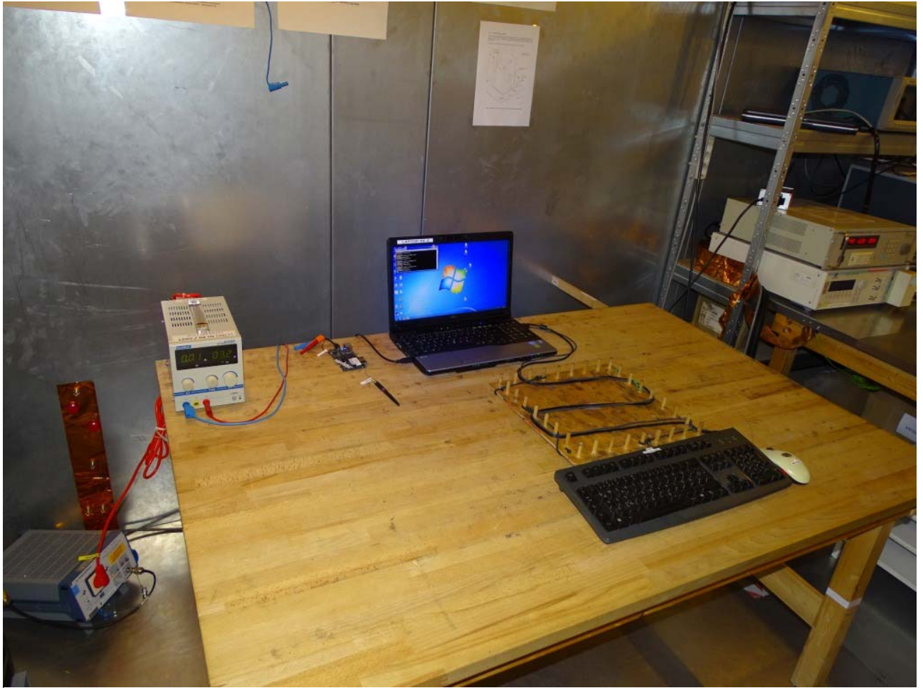
Photo 5: Test setup for conducted measurements at AC port
