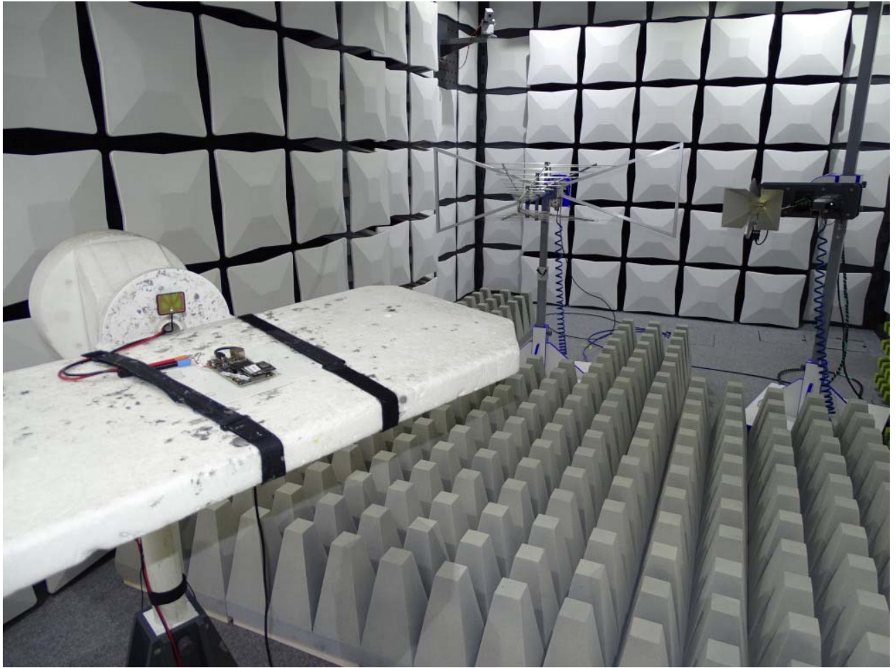
Photo 4: Test setup for radiated measurements in fully-anechoic chamber above 1 GHz
