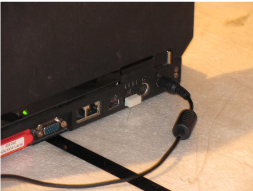
EUT connected to USB port during the radiated emission test.
