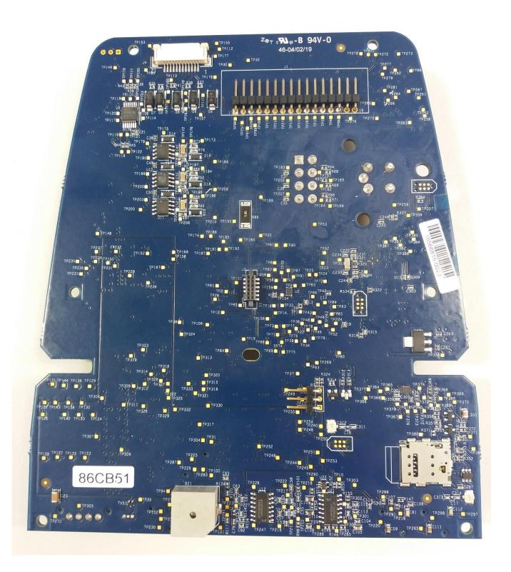
Below is the battery board fitted to the battery compartment that connects the battery and external power to the mainboard.
