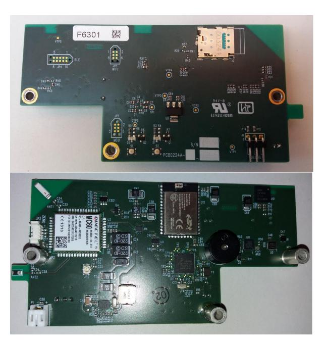
Note that this board is a prototype board so has no test points on the back of the WGM110 and the prototype board numbering (PCB0224A not DM-05002014). Also the BGM123A part is a BGM123N and the bluetooth antenna is still present on the MC60. Additionally production units will omit buzzer BZ1 and one LED and microswitch. However all other components are of the correct type and placement.
