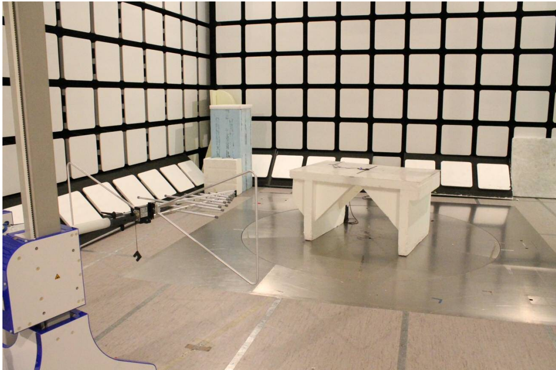
Photograph 1. Radiated Spurious Emissions 30 – 1000 MHz
