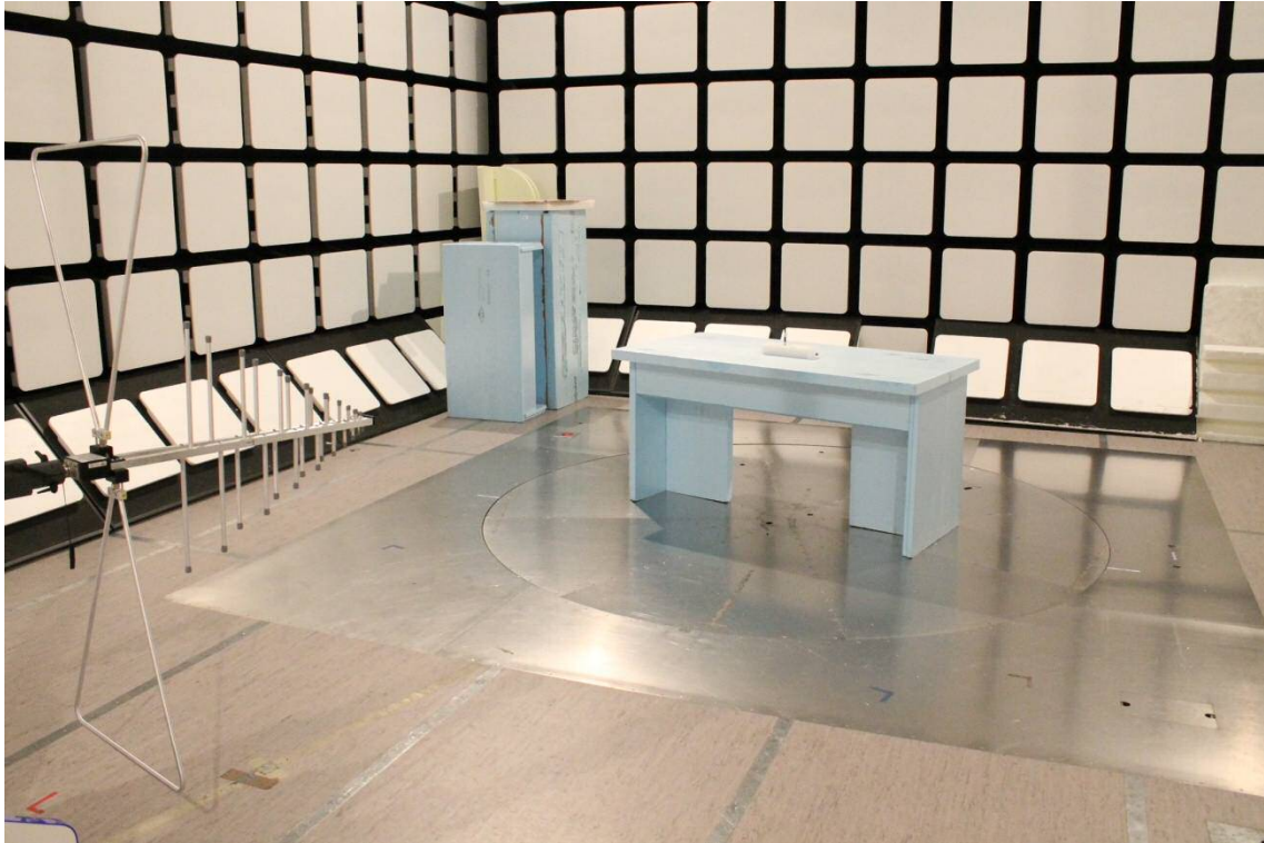
Photograph 1. Radiated Spurious Emissions 30 – 1000 MHz
