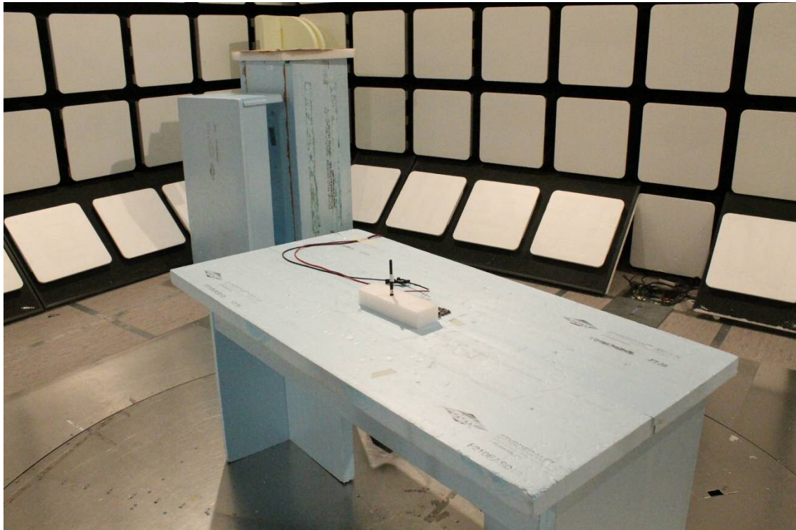
Photograph 3. EUT on table < 1GHz
