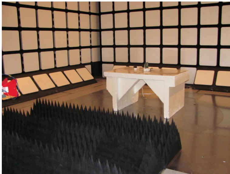
Photograph 4. Radiated emissions 1-18 GHz int. antenna
