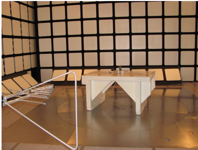
Photograph 2. Radiated emissions 30 - 1000 MHz int. antenna
