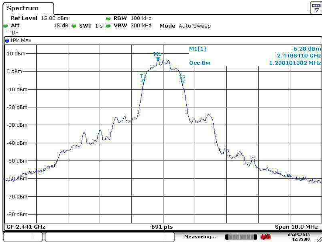
Figure 112. Mid channel 99% Occupied Power Bandwidth (3 Mbps).
