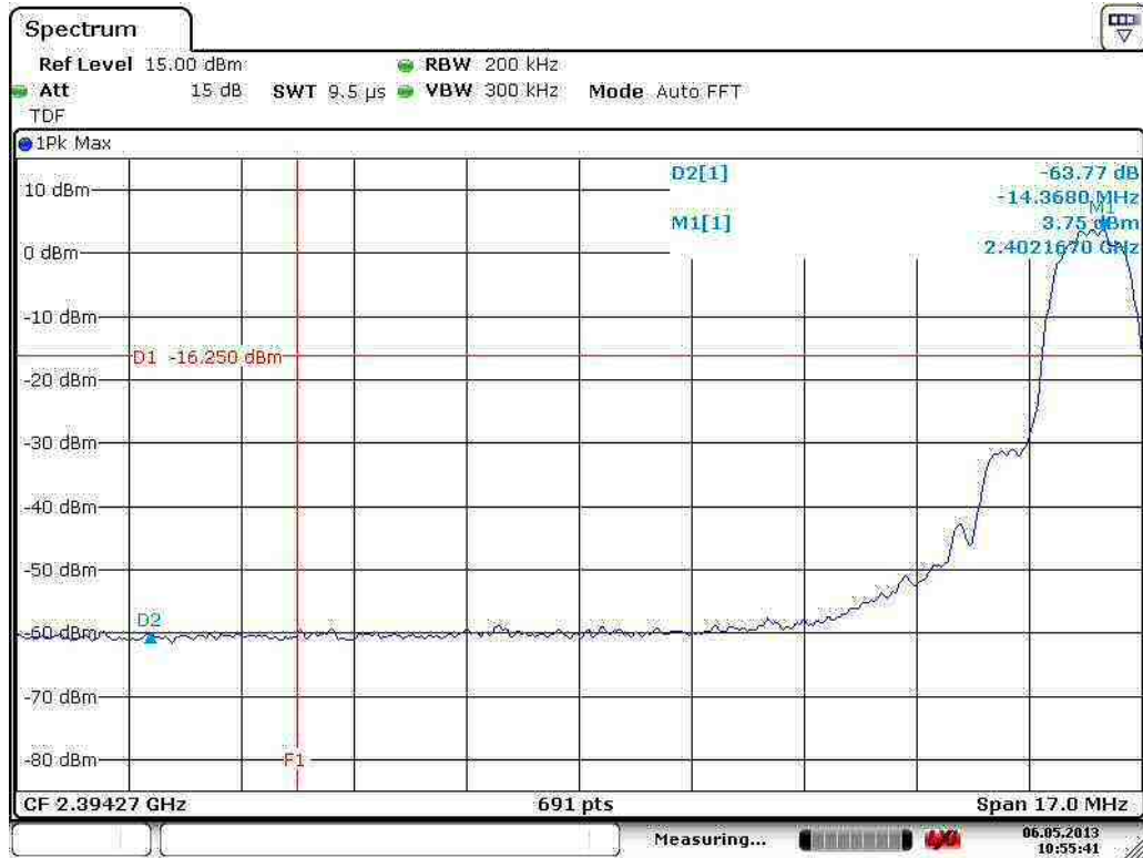
Figure 74. Low channel conductive emission at low band edge (3 Mbps).
