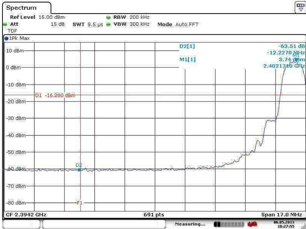
Figure 60. Low channel conductive emission at low band edge (2 Mbps).
