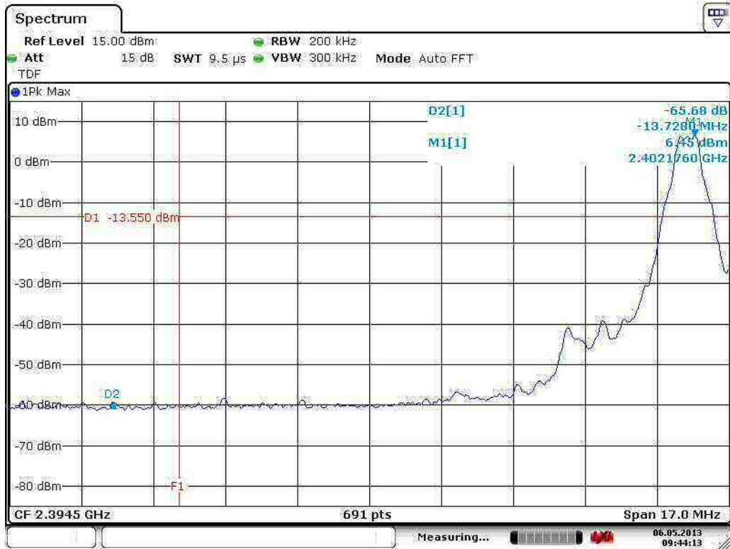
Figure 46. Low channel conductive emission at low band edge (1 Mbps).
