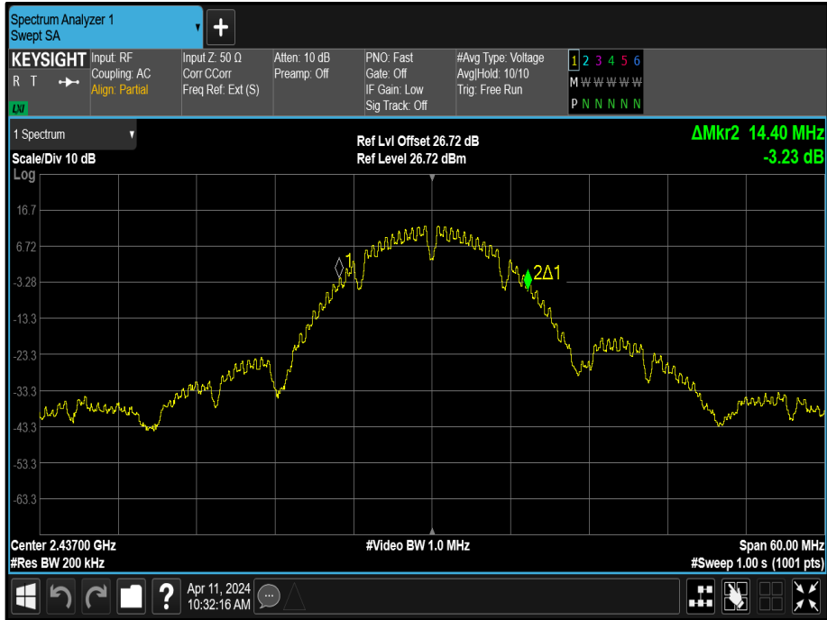
Figure 3 - 2437 MHz (CH6) 99% Bandwidth
