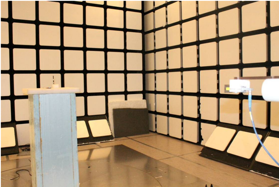
Photograph 3. Radiated Spurious Emissions 18 – 26.5 GHz
