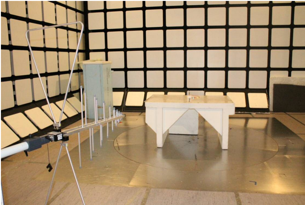
Photograph 1. Radiated Spurious Emissions 30 – 1000 MHz
