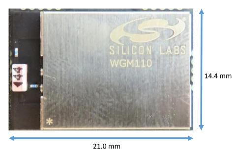
Figure 1: WGM110 External Photo, top view
