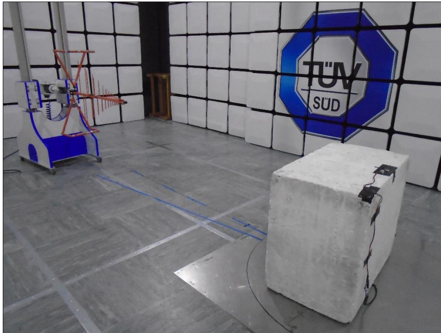
Figure 3 - Test Setup - 30 MHz to 1 GHz - Z
