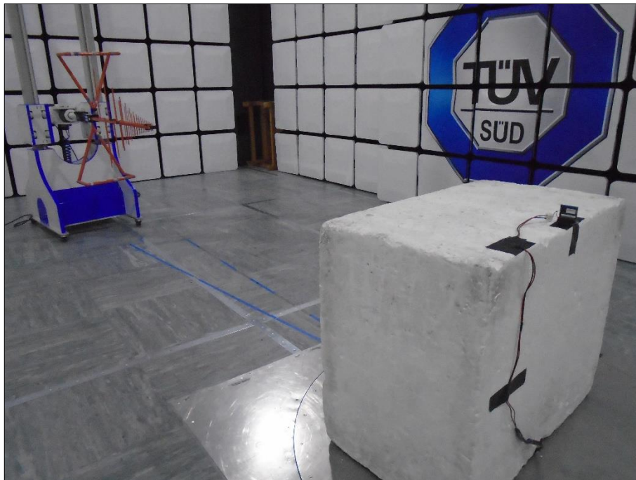
Figure 2 - Test Setup - 30 MHz to 1 GHz - Y
