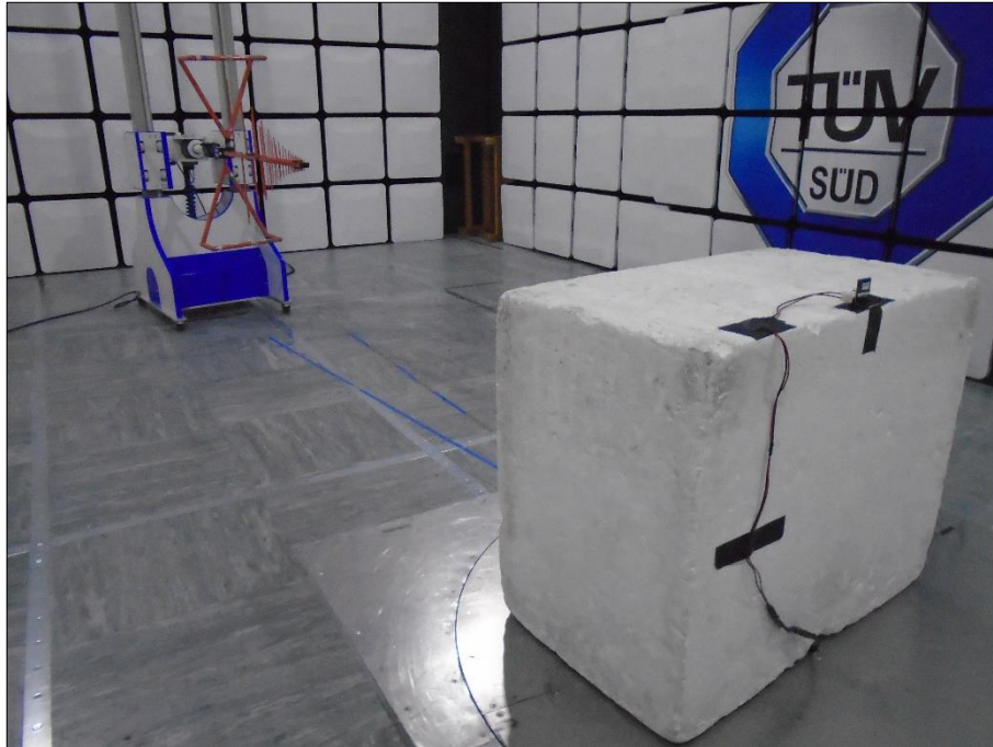
Figure 1 - Test Setup - 30 MHz to 1 GHz - X
