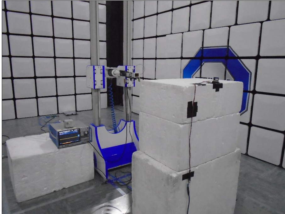
Figure 11 - Test Setup - 18 GHz to 25 GHz - Y
