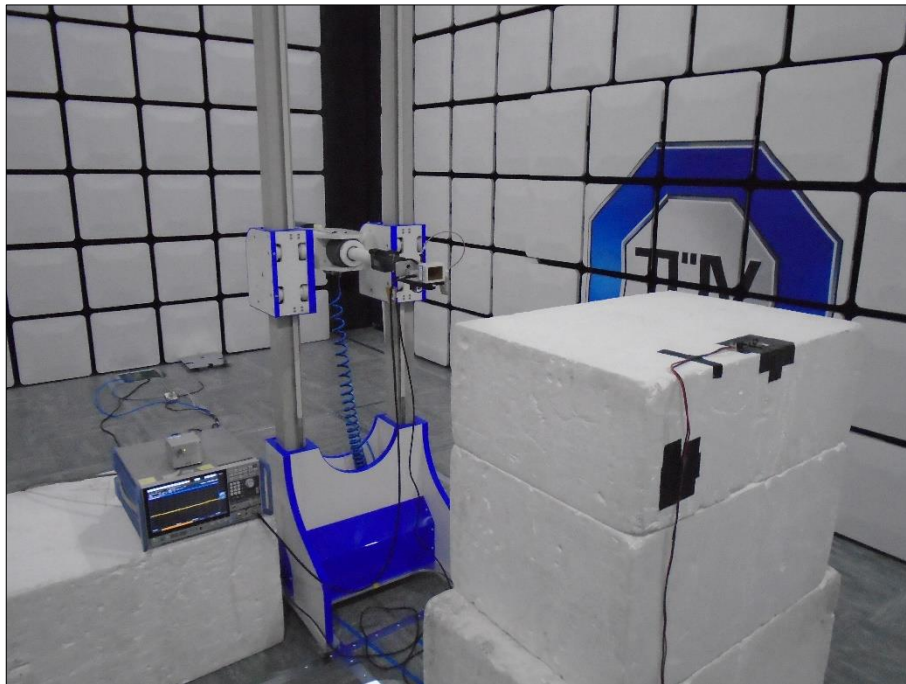
Figure 12 - Test Setup - 18 GHz to 25 GHz - Z
