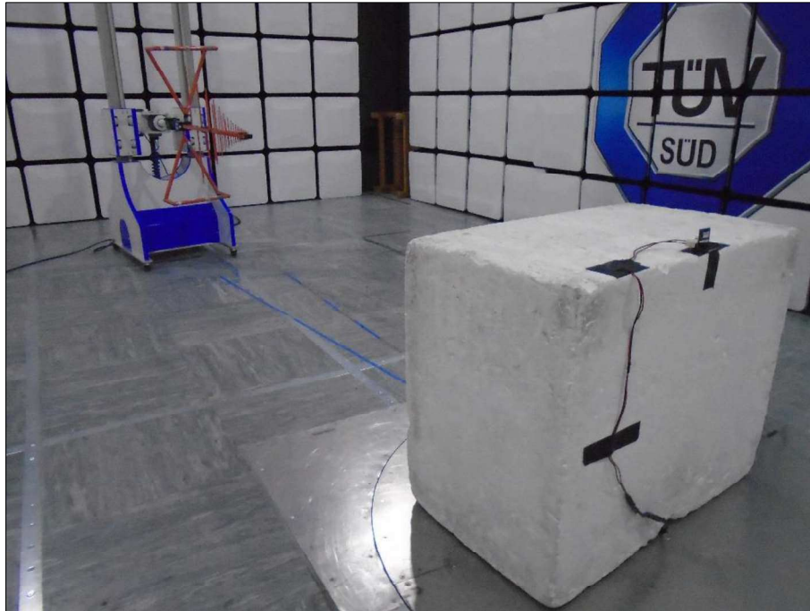
Figure 137 - Test Setup - 30 MHz to 1 GHz - X
