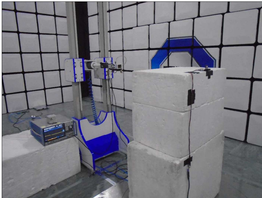
Figure 146 - Test Setup - 18 GHz to 25 GHz - X
