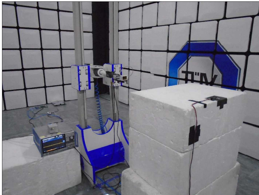
Figure 148 - Test Setup - 18 GHz to 25 GHz - Z
