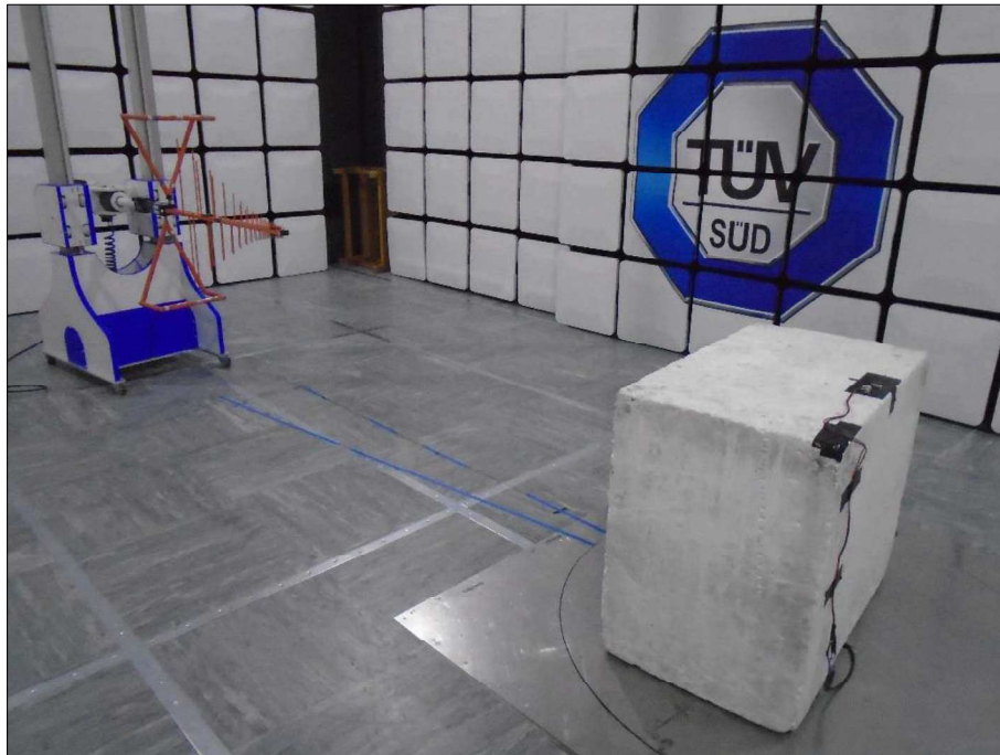
Figure 139 - Test Setup - 30 MHz to 1 GHz - Z
