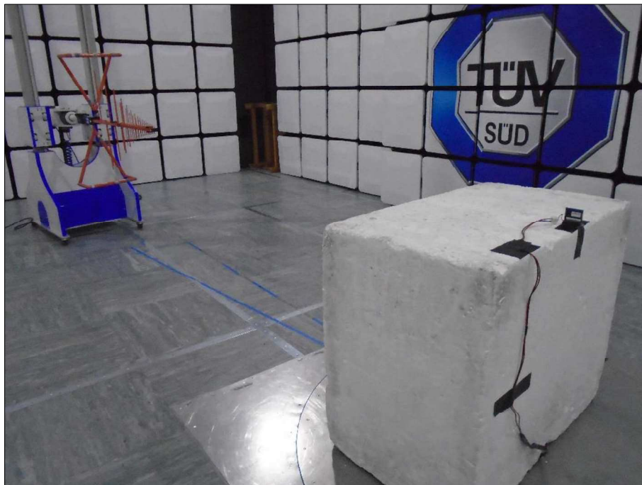
Figure 138 - Test Setup - 30 MHz to 1 GHz - Y
