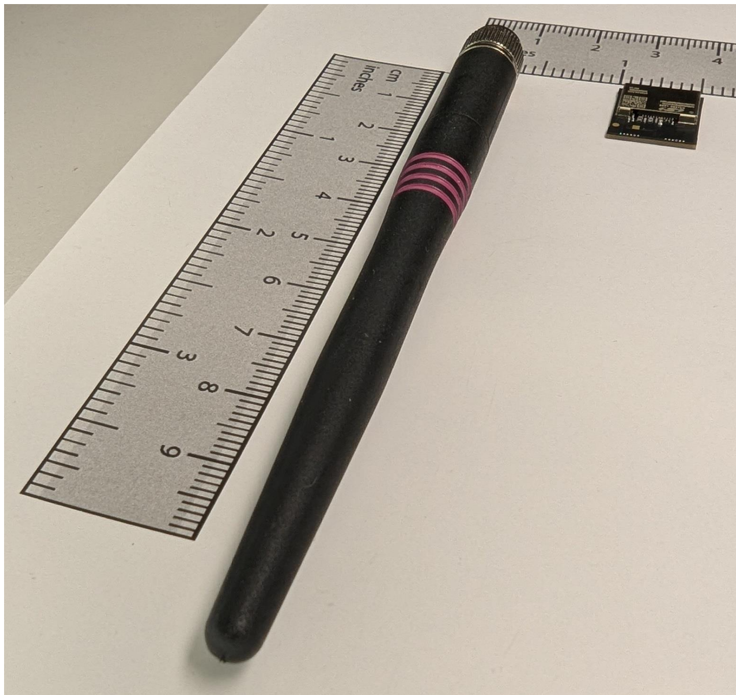
Figure 4: Reverse Vertical/Oblique Full View of the Reference External Antenna, next to the MGM260P32N Module
