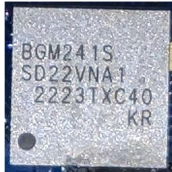
Figure 1: Top/Front External View of a BGM241S22A Engineering Sample (Dimensions: 7 mm x 7 mm x 1.18 mm – Fully Representative of the Production Modules)
