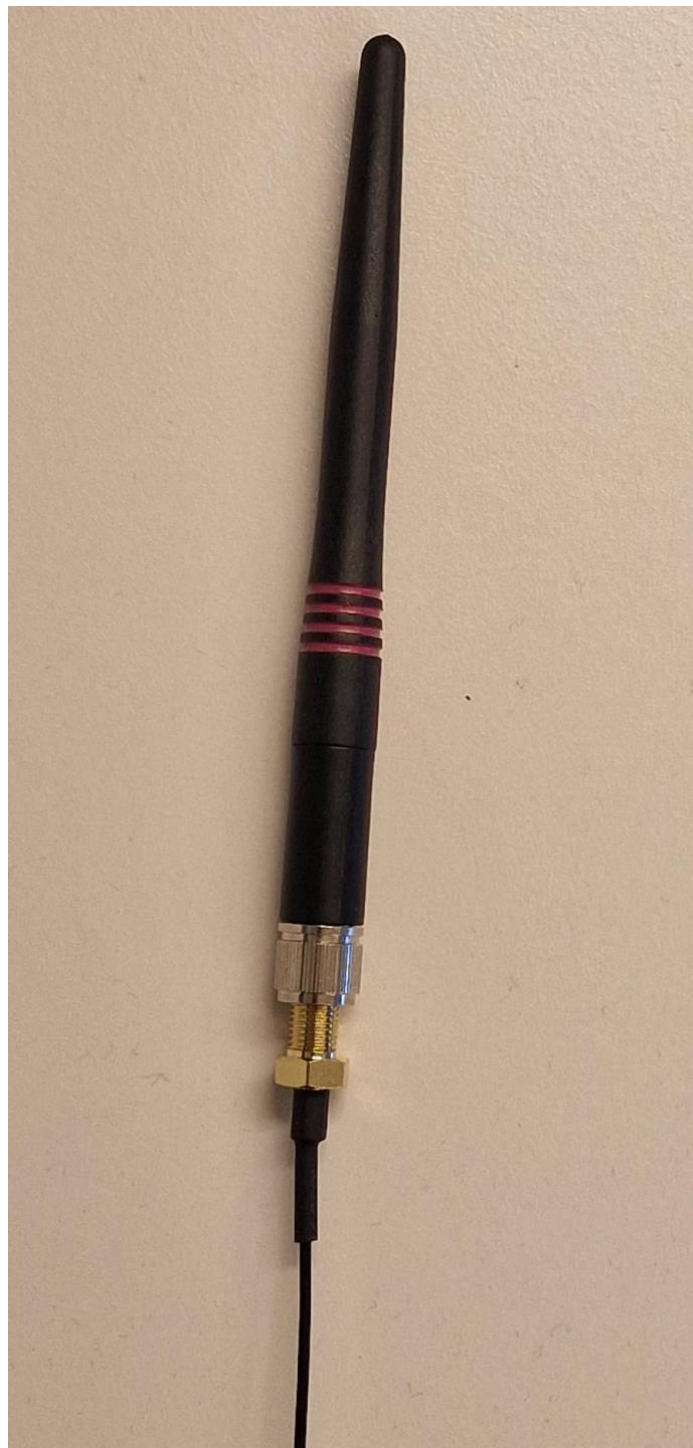
Figure 3: Detail of the External Antenna and the IpeX Coaxial Cable, Belonging to the Complete Reference Antenna Subsystem for the MGM240P32N Module
