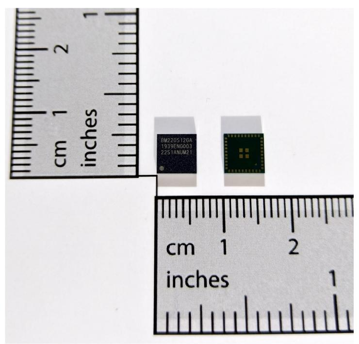
Figure 1: Top/Front and Bottom/Rear External View of BGM220S12A
