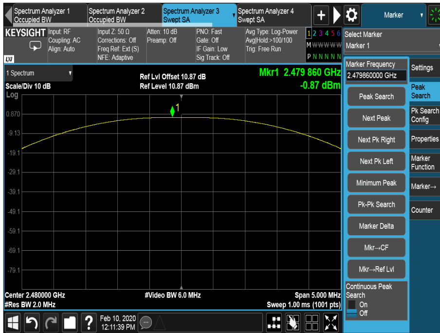
Figure 3 - 2480 MHz - Maximum Output Power
