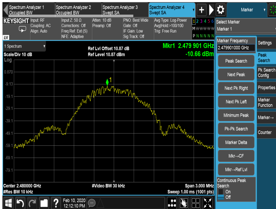
Figure 15 - 2480 MHz - Power Spectral Density
