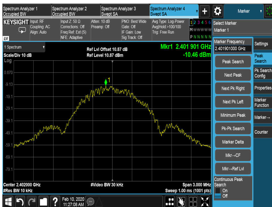
Figure 13 - 2402 MHz – Power Spectral Density
