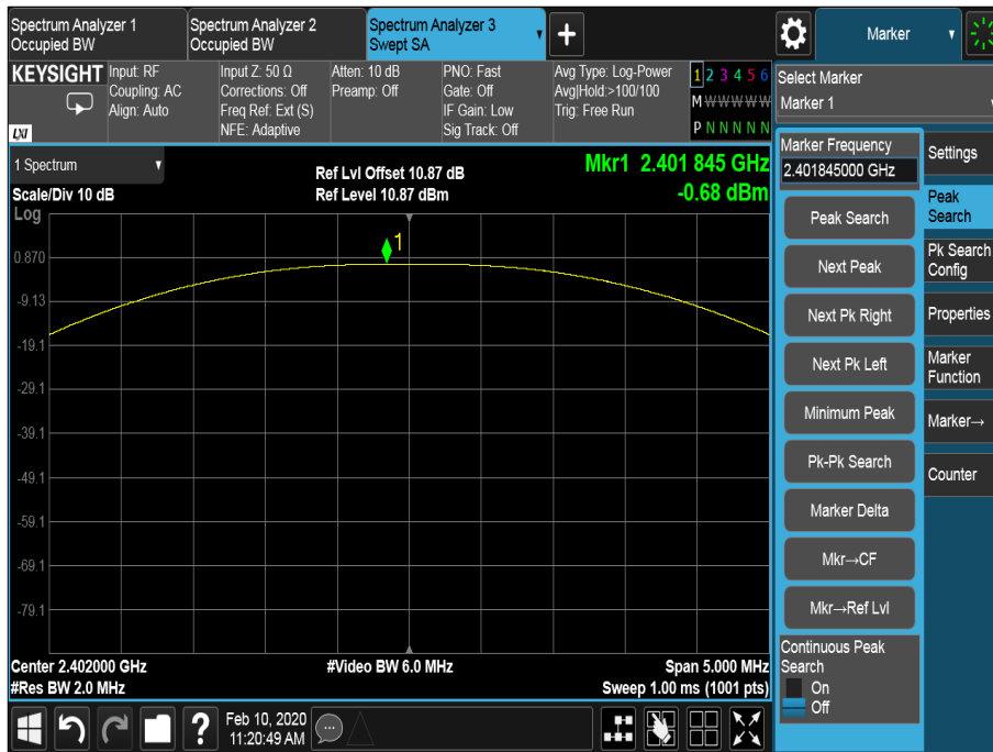
Figure 1 - 2402 MHz - Maximum Output Power
