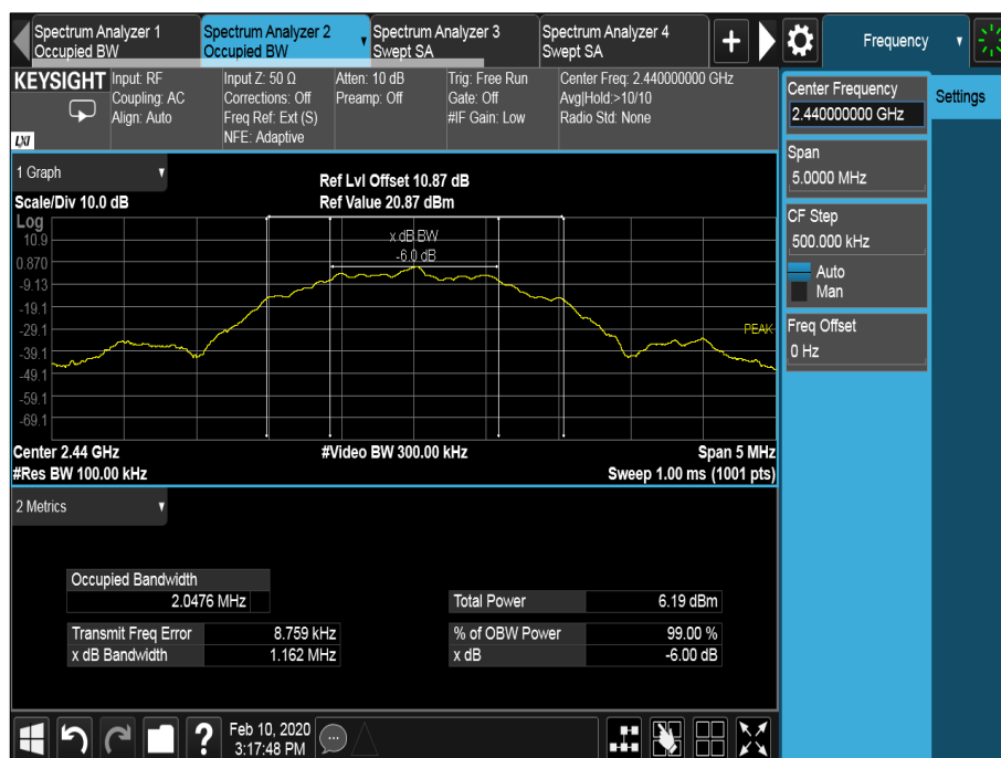
Figure 11 - 2440 MHz – Emission Bandwidth
