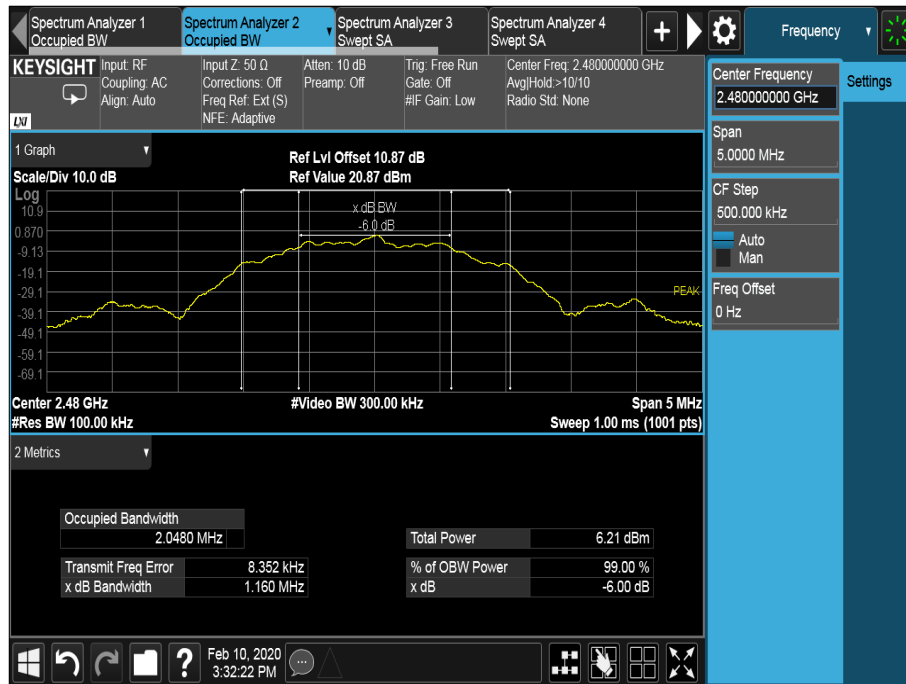
Figure 12 - 2480 MHz – Emission Bandwidth
