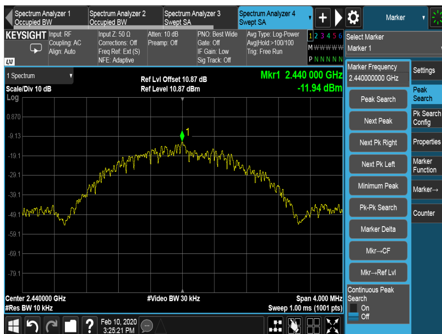
Figure 17 - 2440 MHz – Power Spectral Density
