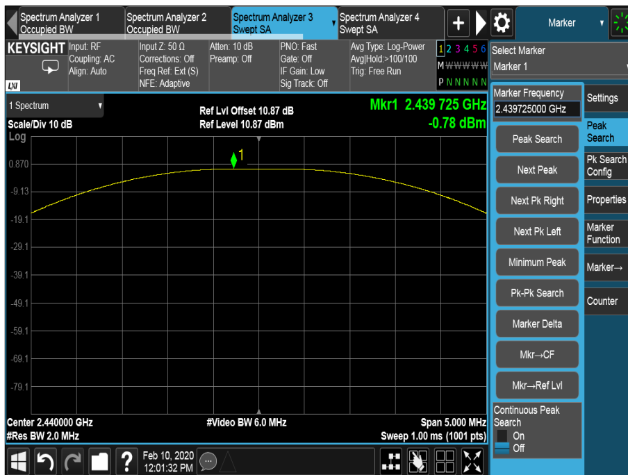
Figure 2 - 2440 MHz - Maximum Output Power
