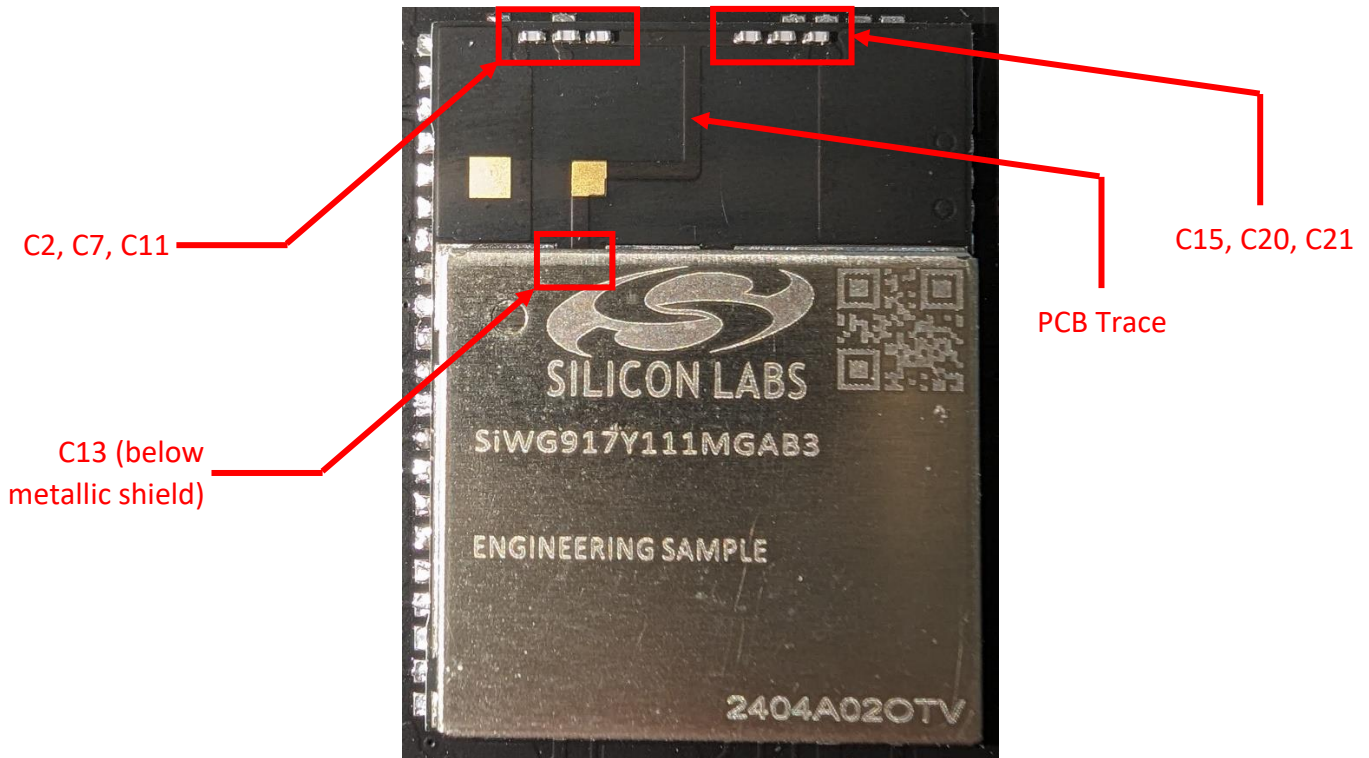
Figure 6: Photo of the antenna realized on the SiW917Y1GA module. It consists of a PCB antenna trace and 7 ceramic capacitors (C2, C7, C11, C13, C15, C20 and C21).
