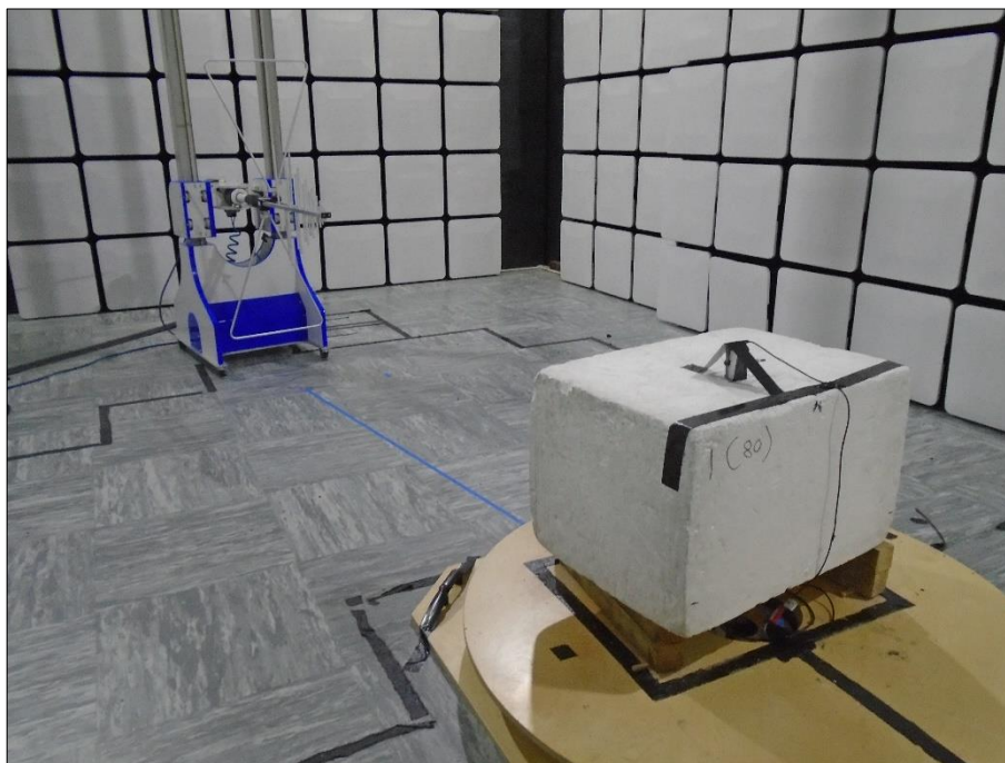
Figure 141 - Test Setup - 30 MHz to 1 GHz Y Plane
