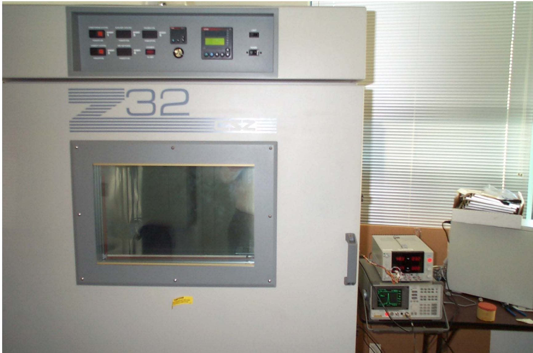
Figure 4. Frequency Stability Test Set-up – temperature chamber door closed
