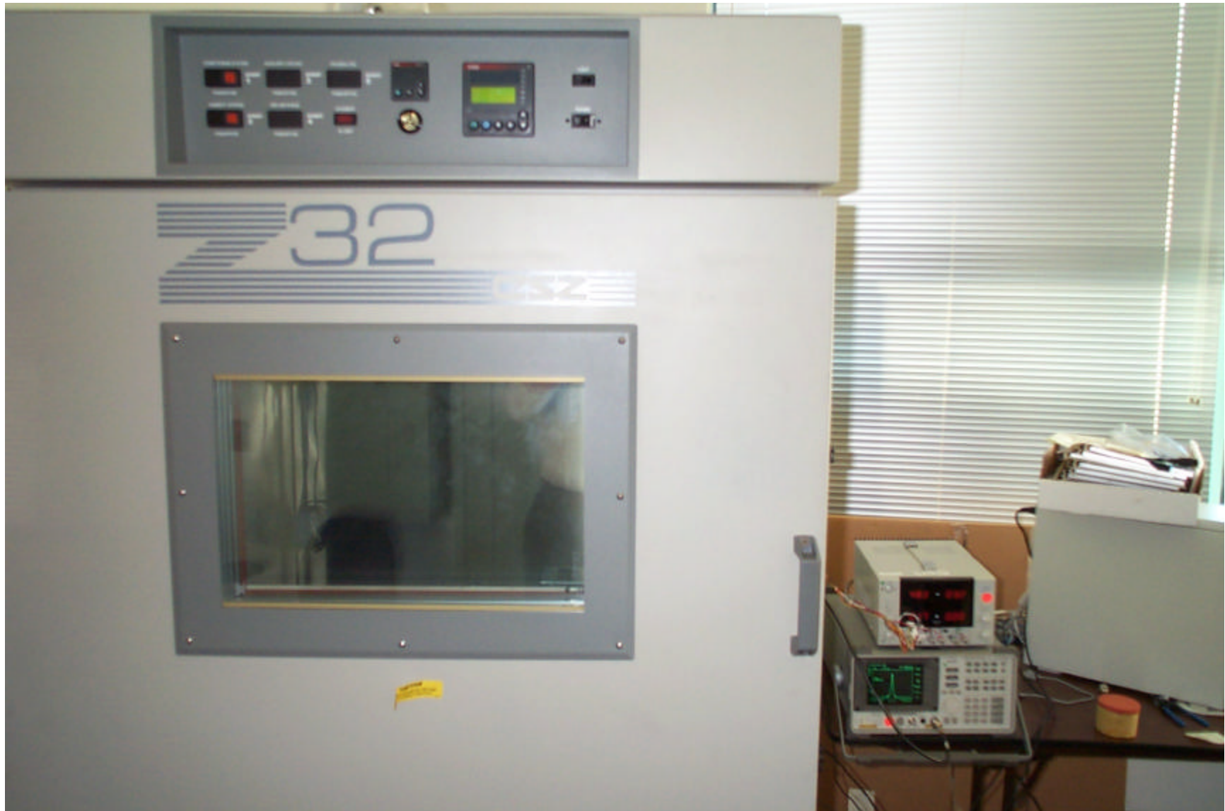
Figure 5. Frequency Stability Test Set-up – temperature chamber door closed
