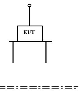
Separation distance = 3 meters Receive antenna varied 1-4 meters EUT placed on OATS on wooden table above ground reference plane.
