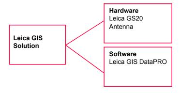
The Leica Geosystems GIS DataPRO office software is comprised of a GPS post-processing system and data editing functionality which works in the native ESRI shape-file format.
