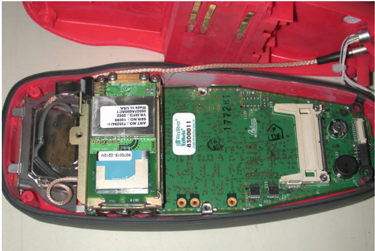
Photo 2 Detail View – Unit opened – bluetooth module shown
