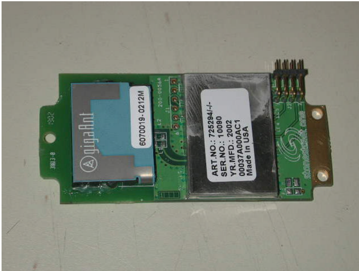
Photo 4 Detail View – Bluetooth module – Top
