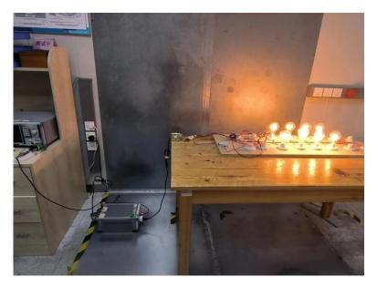
Radiated Emissions From 30MHz-1000MHz
