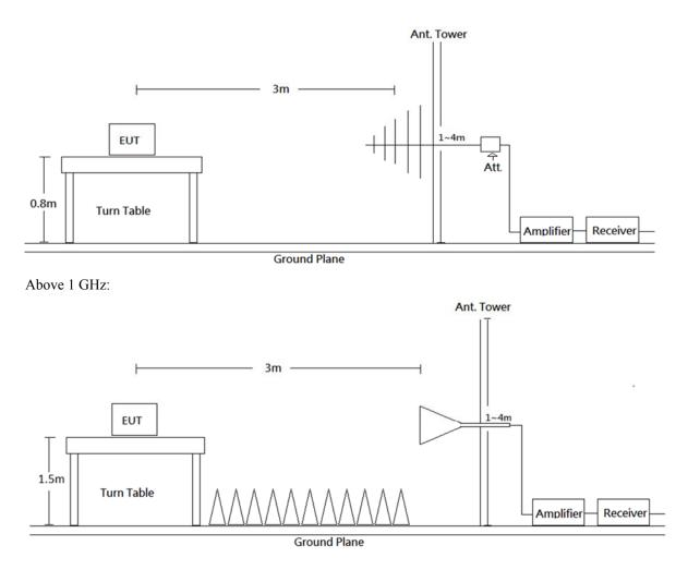
Radiated emission tests were performed in the 3 meters chamber test site, using the setup accordance with the ANSI C63.10-2013. The specification used was the FCC 15.205, FCC 15.209, FCC 15.249 and RSS-GEN, RSS-210 limits.
