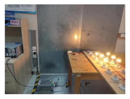
Radiated Emissions From 30MHz-1000MHz
