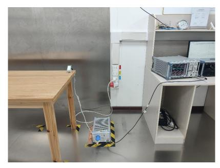
Radiated Emissions From 30MHz-1000MHz
