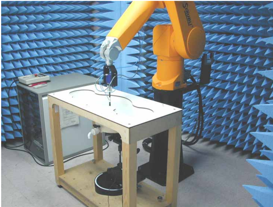
Fig.1 Photograph of the SAR measurement System
