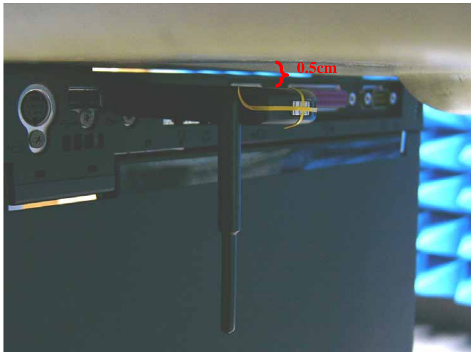
Fig.6 Photo of the Bottom face of the notebook is paralleled with flat Phantom, Antenna is in Vertical direction and Spacing between EUT and phantom – In contact (0.5cm)
