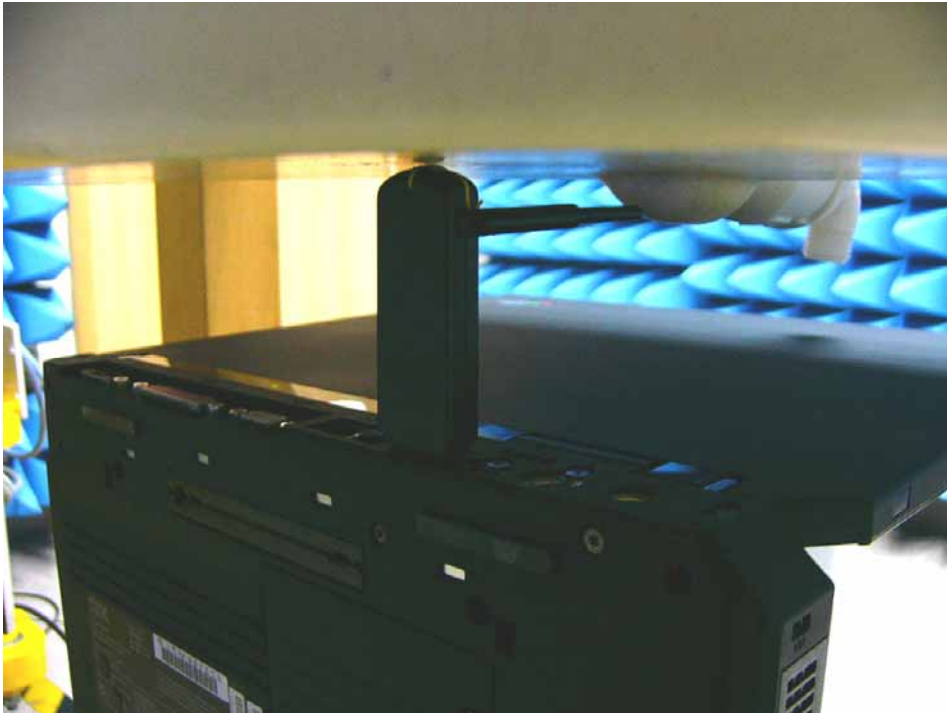
Fig.3 Photo of the Notebook and the top of EUT contact to the Flat phantom, Spacing between EUT and phantom –In contact (0mm)
