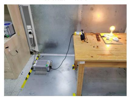
Radiated Emissions From 30MHz-1000MHz
