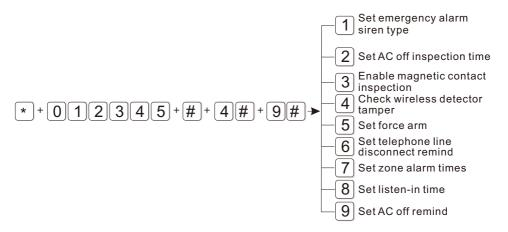
6.4.9.1 Set emergency alarm siren type (the default setting is mute) For example: set emergency alarm siren type is pedal point.
