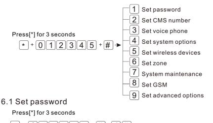
Then operate according to the voice prompt as below. Set password ■)) [1]Set Admin password ■))[2]Set user password Enter password, Please enter the serial number press confirm key to save, of your modified password, confirm press back key to exit. key to confirm, press back key to exit press confirm key to save, **◄**)))The setting is saved Enter password, press confrim key to save, Press back key to exit ■)) The setting is saved
