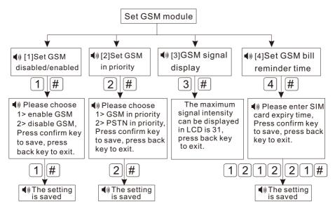
Hint: The alarm control panel will send SMS to cellphone as preset and remind you to recharge as you set GSM bill reminder time before or after ten days.
