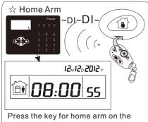
Press the key for home arm on the remote or "HOME"key on the keypad, then you will hear "system stay" And it display home arm icon on the LCD screen.
