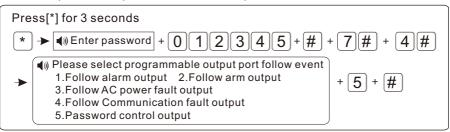
Hint: when setting as password control output, press key 5 for 3 seconds, then enter the user password, the programme output port will be open or closed. Voice phone or SMS also can open or close the outport.
