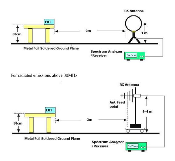
5.2.5. EUT Operation during Test
