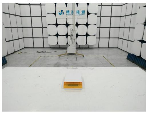
RADIATED EMISSION TEST SETUP ABOVE 1GHz
