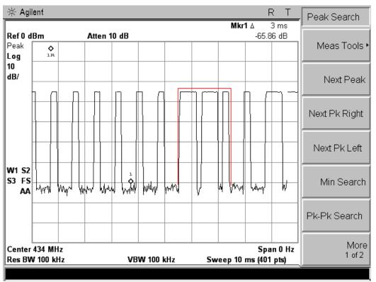
Note: In the red curcle 1, 2 and 3 the gap between long/short impulses is too short, so the analysis can't sweep it clearly continuously. The above 1, 2 and 3 clearly show it. In the red curcle 1 it includes one long impulses and one short impulses. In the red curcle 2 it includes four long impulses and one short impulse. In the red curcle 3 it includes two long impulses and one short impulses.
