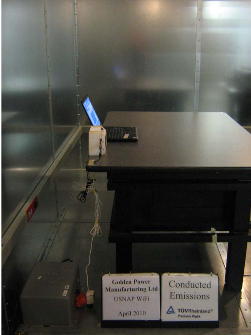
Figure 11: Photo of Test Setup for USNAP WiFi Module, AC Conducted Emission (Side View)
