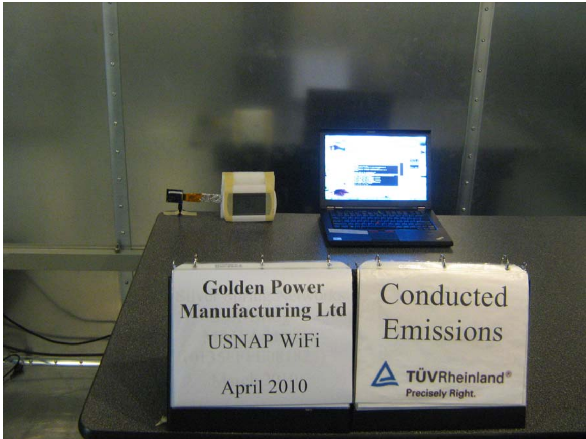
Figure 10: Photo of Test Setup for USNAP WiFi Module, AC Conducted Emission (Front View)
