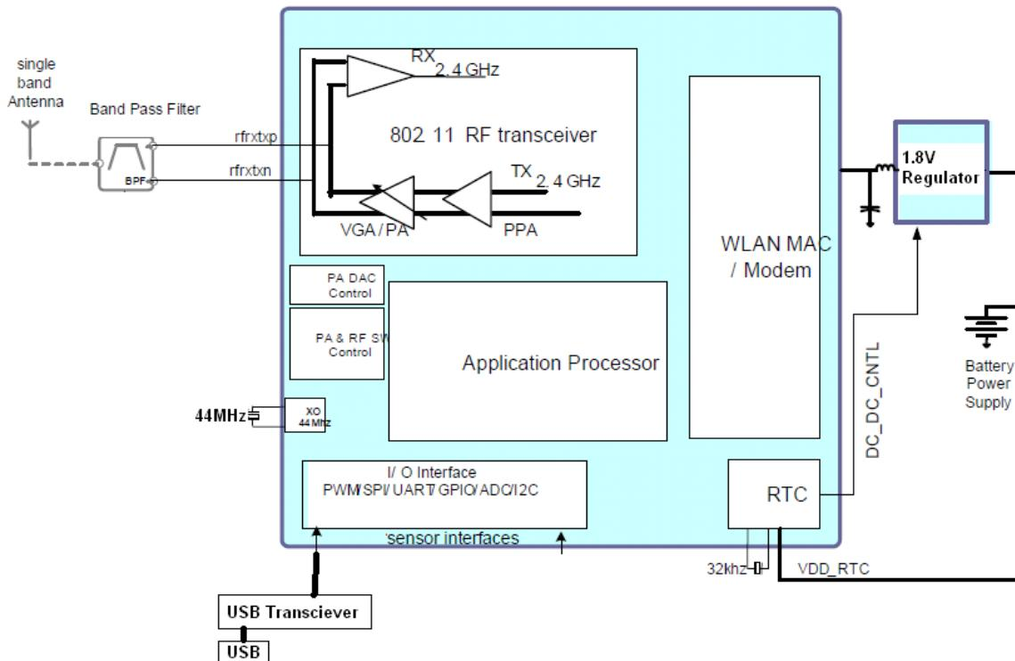
The GS1011 is a single chip system on chip solution that includes an internal 2.45GHz RF transceiver which is IEEE 802.11b/g – compatible and supports direct sequence spread spectrum (DSSS). It supports BPSK/QPSK/CCK modulation with data rates up to 11 Mb/s (802.11b).
