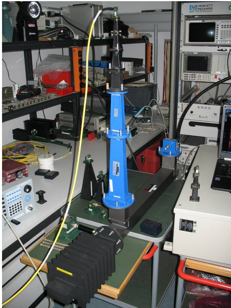
Photo No. 7: conducted measurements, spurious emissions up to 40 GHz
