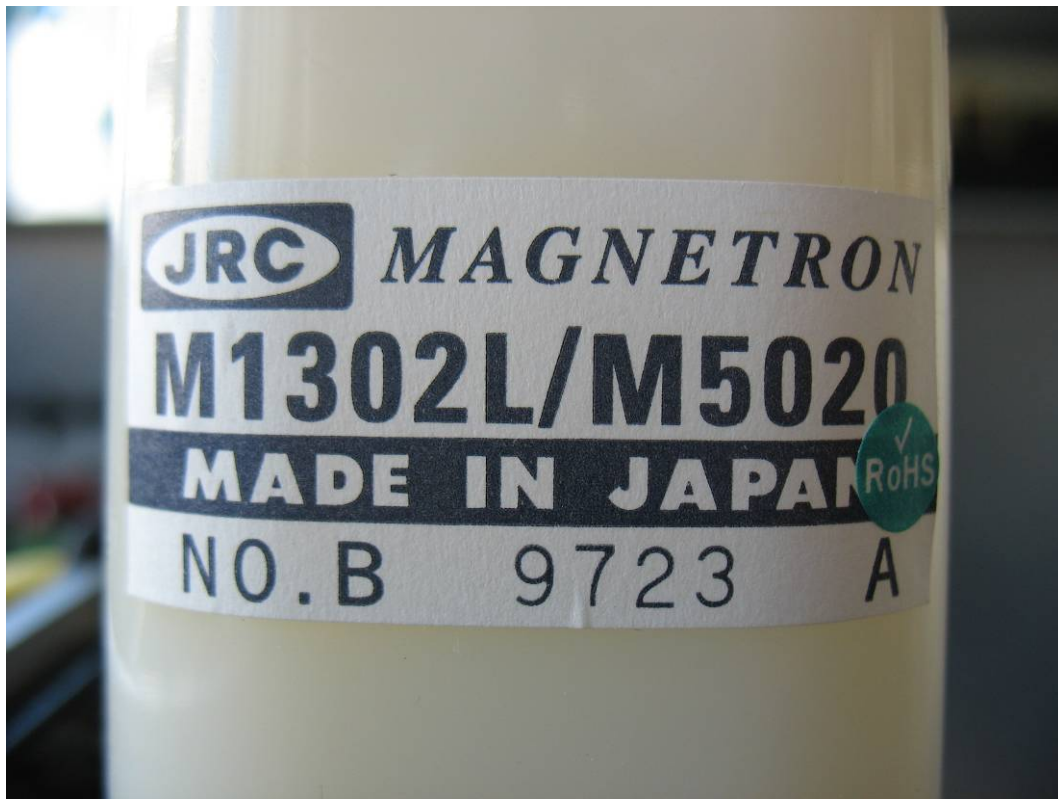
Photo No. 3: 30 kW Magnetron, type label
