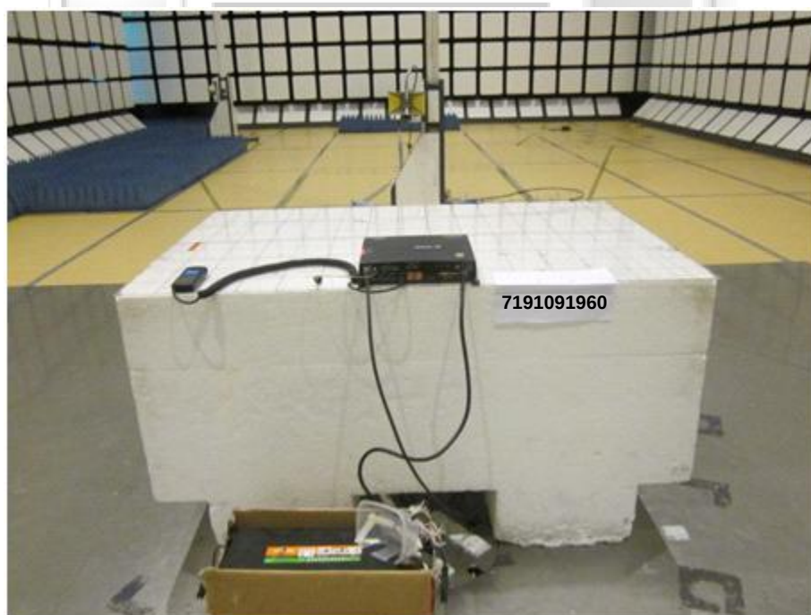
Radiated Emissions Test Setup (Rear View)
