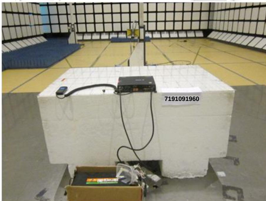
Band Edge Compliance (Radiated) Test Setup
