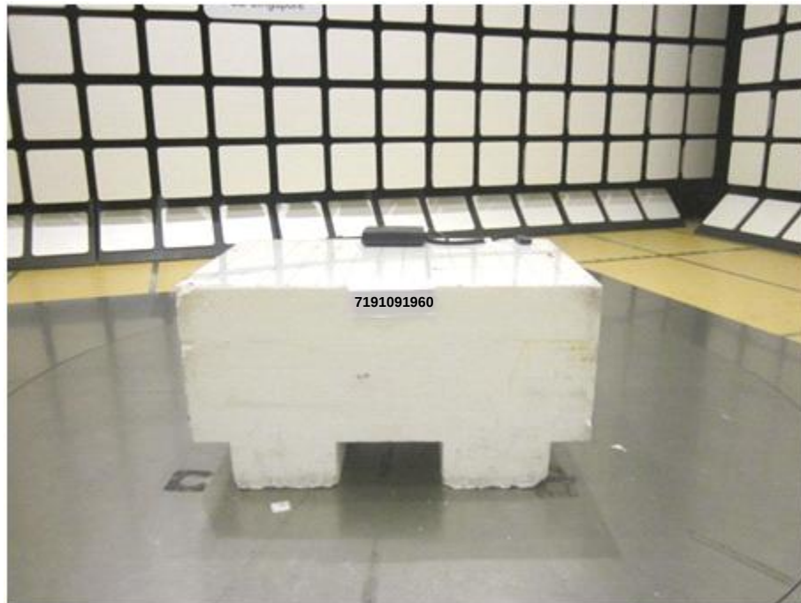
Radiated Emissions Test Setup (Front View)
